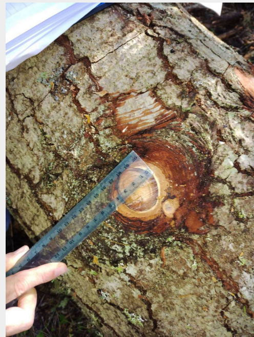
Fig. 3 - Measuring the knot size of Silver fir trunks using a ruler.
