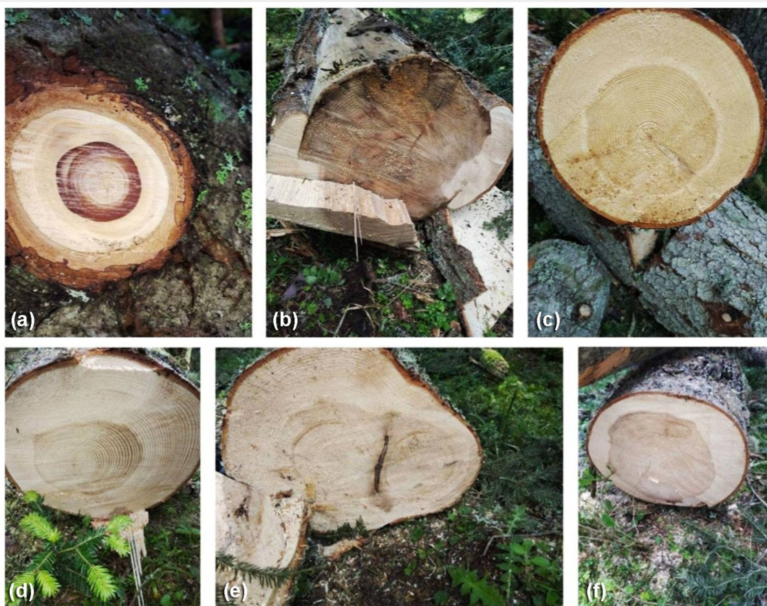
Fig. 5 - Some of the recorded wood defects: knot (a); damage caused by mechanical influences and rot (b); wet heart (c), pith eccentricity and compression wood (d), double heart and ingrown bark (e); ellipticity (f).
