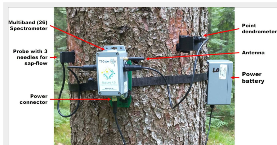
Fig. 1 - TreeTalker's components. Credits: Antonio Tomao. Modified by the authors.
