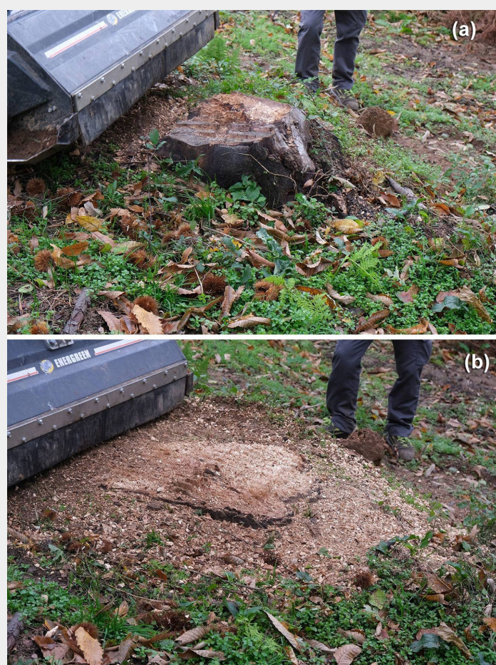
Fig. 3 - One of the test stumps before (a) and after (b) grinding.
