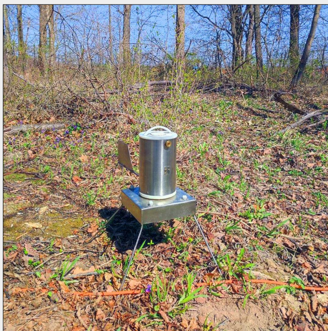
Fig. 2 - Automatic volumetric spore trap (AMET, Velké Bílovice, Czechia), installed to sample the air 30 cm above the ground in an unmanaged mixed forest infected with the sooty bark disease.
