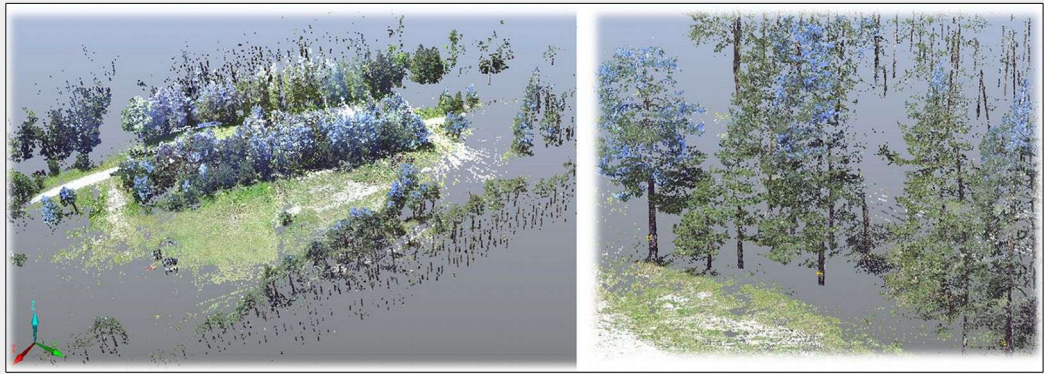
Fig. 5 - Result of the registration of the 8-point clouds.
