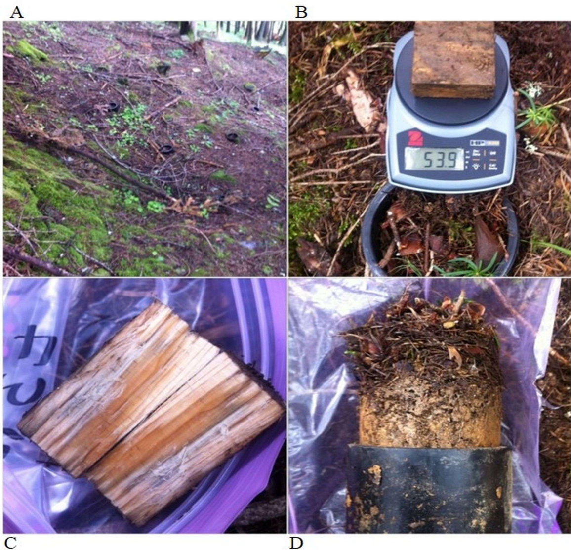
Fig. S2 - Example of the destructive in-field mesocosm sampling (wood and soil). (a) Study site (N1); (b) weighing of the collected Picea abies wood block; (c) cross-section of the wood block after 52 weeks (July 2014) of decomposition; (d) sampling of the mesocosm soil (0-5 cm).
