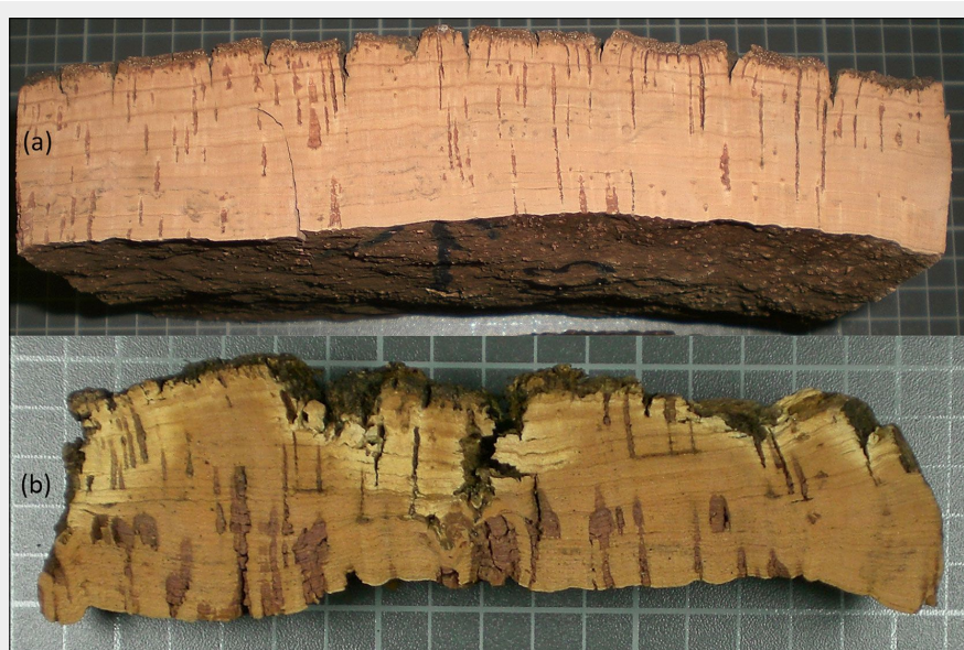
Fig. 1 - (a) Piece of cork classified as highest visual quality (HQ); (b) piece of cork with yellow stain clearly present (YS).
