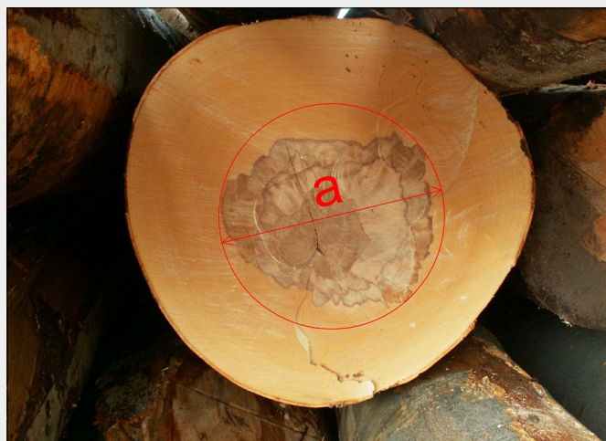
Fig. 2 - Measurement of red heartwood as the diameter of the circle of the contaminated area ( a ) at the thicker end of assortments.
